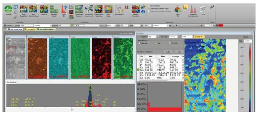
Quantification of segregating element concentrations is determined against a range of reference steel standards using linear regression, providing accurate quantitative results. Typical calibration curves for different segregating elements of interest are displayed below.
