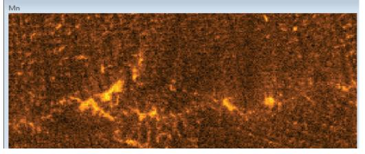
The ATLAS not only provides visual evidence of macrosegregation in elemental maps, but quantitative measurement of elemental concentrations in the centerline region of continuously cast billets and slabs.
